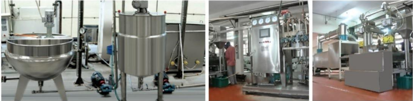
化糖锅和储糖锅 Sugar dissolving cooker and storage tank 真空薄膜熬糖机组 Candy micro-film vacuum cooking unit 浇注机 Depositing machine
