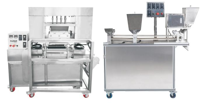
Application: Can produce two-color and sandwich pearl small taro round machine, two-color and sandwich cylindrical large taro.
