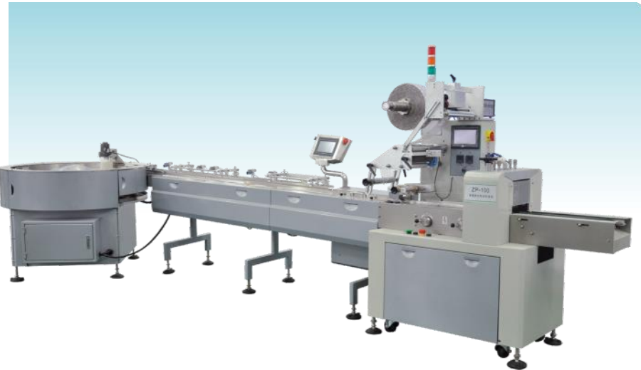
SN-350高速枕式包装机 Fast Pillow Packing Machine
